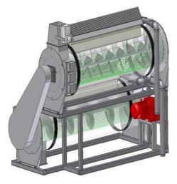
Reducing kW/ton from the Preparation of Raw Material - The online optical monitoring of raw material properties combined with indirect heat and external condensing unit for moisture removal allow the chemical properties within the material to be brought to an ambient structure for the production of a pellet.
